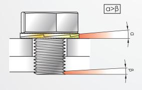
In each group, there are different serrations on the top and bottom. The large sawtooth has an inclination  $\,\alpha\,$  larger than the bolt thread angle  $\,\beta$  .
