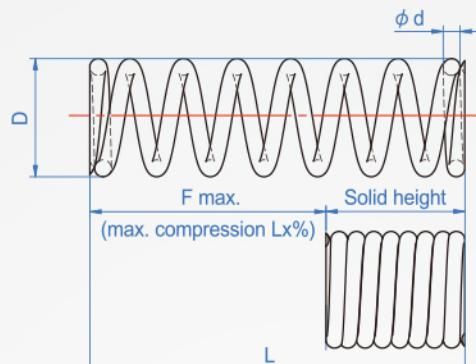
◆ D Tolerance : Below  $\phi 16$  +0 -0.5mm
